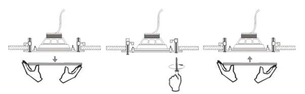
Once the hole is cut, remove the protective metal grille and insert the speaker in the hole. And make sure the fastening hooks are unscrewed. Tighten the fastening screws in a clockwise direction until the speaker is locked.
